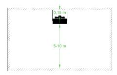
In case of higher heat demand, more units can be installed in the room. In order to ensure proper air flow, it is necessary to maintain the recommended distances between the heaters, as shown in the following figure.
